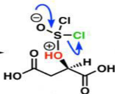
Expulsion of Cl - to form protonated chlorosulfite
